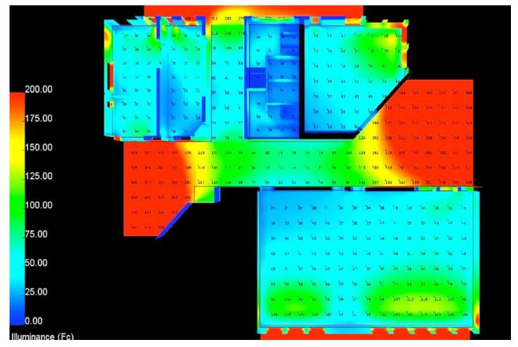
Computer drawing of light intensity in Archbold's Learning Center. Even blue green shading in interior rooms shows desirabl levels. Reds and yellows are brightly-lit exterior decks.
